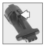
This adapter may be included with your vehicle as part of the heavy-duty trailer wiring package.
